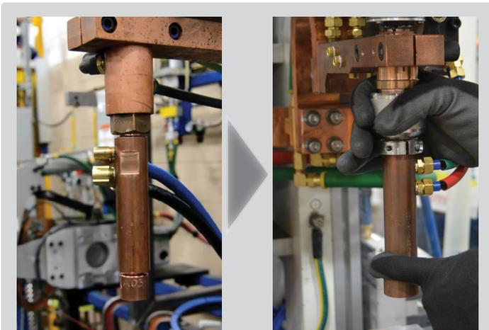
Easily retrofit your existing adapter assembly (left) with the Quick Change Electrode (right).
